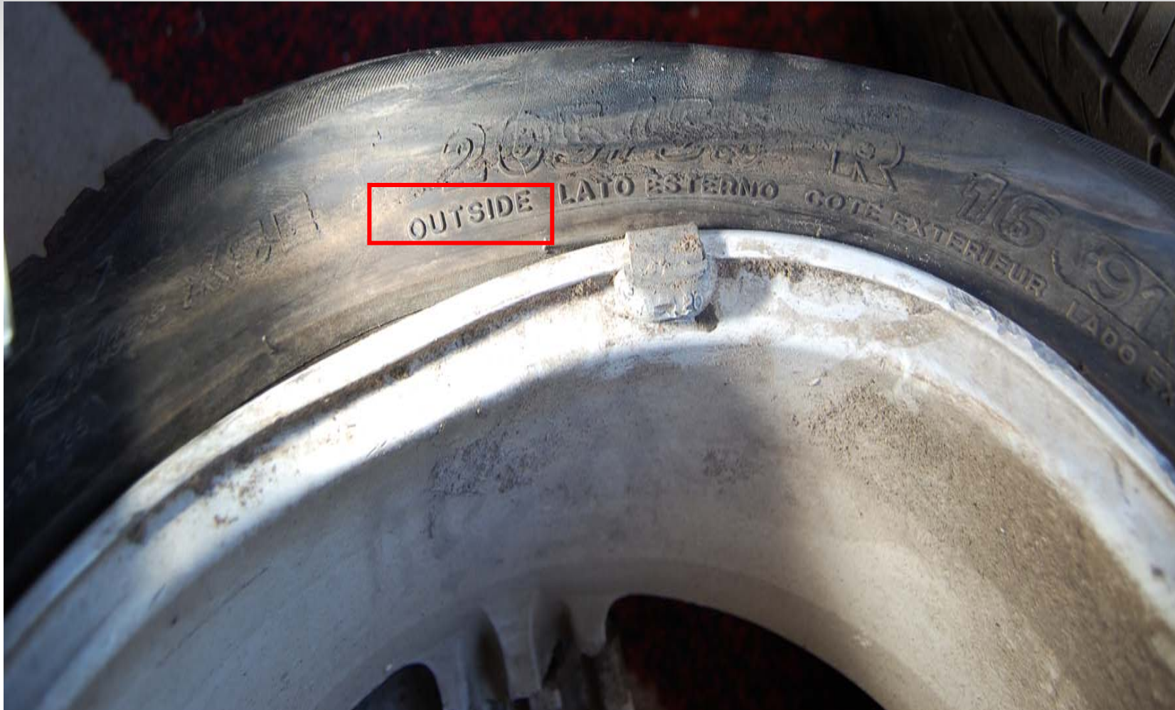
ALL 4 OF THE NISSAN'S TIRES WERE LABELLED "OUTSIDE" ON THE INTENDED OUTSIDE OF THE TIRE
